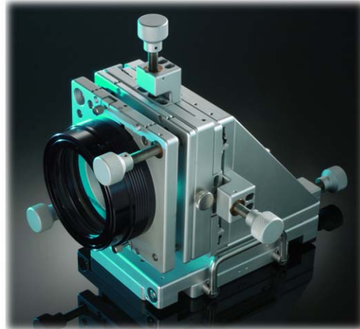
Horizontal, 7-Axis Stage with Bayonet Mount and Transmission Sphere
